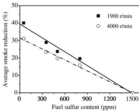
Fig. 2. Smoke reduction and fuel sulfur content.
