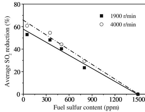
Fig. 8. SO<sub>2</sub> reduction and fuel sulfur content.
